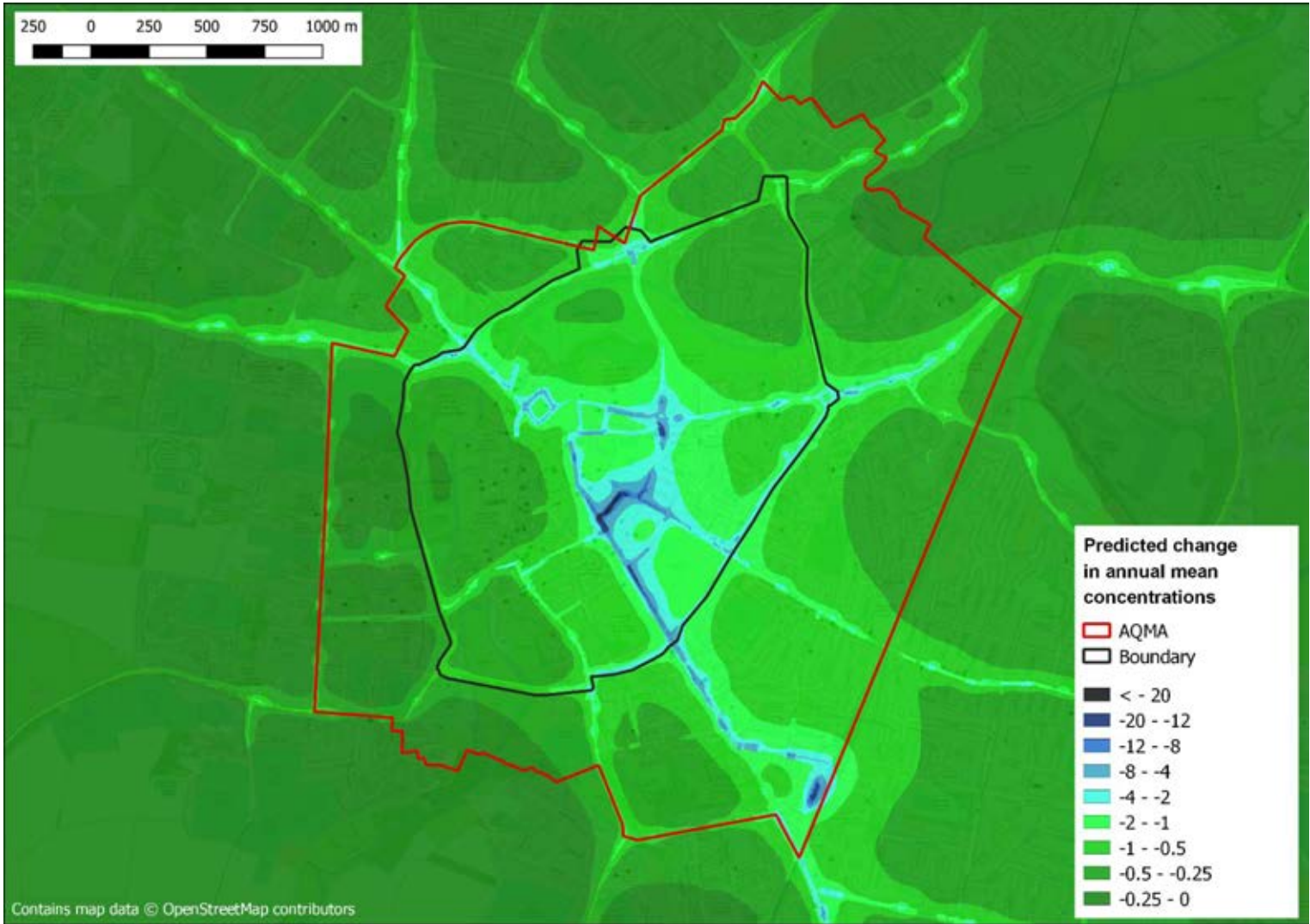
Figure 13: Predicted change in annual average NO 2 concentrations with the implementation of the non-CAZ intervention package, central Cambridge, 2021, \mu\text{g.m}^{-3}
